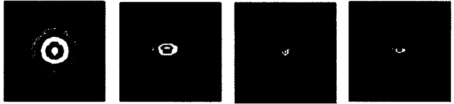
FIGURE 6. Fabrication of a nanolayered GRIN lens (left, top) is CMOS compatible. Mode and spot sizes (above, from left to right) are compared for single-mode fiber ( 8 \times 8 \mu\text{m} ); wedge fiber ( 3 \times 8 \mu\text{m} ); a super-GRIN lens ( 0.9 \times 2 \mu\text{m} ); and a laser diode ( 1 \times 3.5 \mu\text{m} ). Super-GRIN lenses serve to couple light from fibers in V-groove arrays into planar nanowaveguides (left, bottom).
